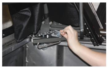
When retracted, two chains hold the canopy inside the shroud so it does not slide out while driving. The chains are placed over the tall ends of the catch.
