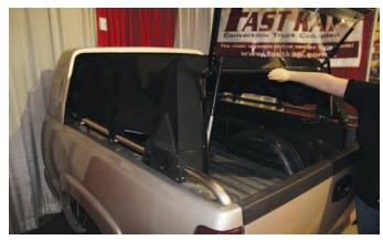
Push the canopy back slightly making sure the fabric tucks into the folds created as the bows collapse. The canopy slides with a slight push of your hand. There is plastic stitched into the flaps but it is split in the middle between each bows so it folds properly and stays flat when driving on the highway when extended. Its best to push from the middle for the easiest sliding action but it can be pushed from each side as well.
