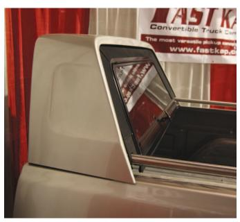
The canopy now fully collapsed inside the shroud. To deploy the canopy, simple lift the glass, unlatch the chains and with one hand from the side of the truck pull the canopy out. Reattach the catches and snap the handles in place, the sides can then be folded down and snapped into place.
