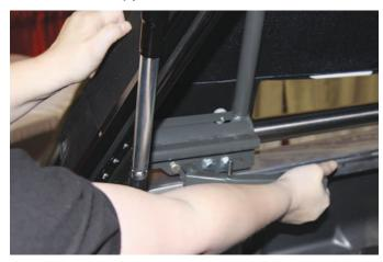
Reach inside and pull the clamp handle towards the rear of the cap this releases the spring tension on the fabric and the canopy may slide forward slightly when you pull the handle.
